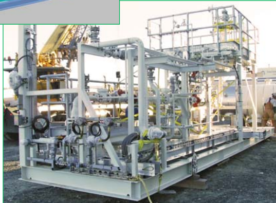
Digital design tools help us visualize, plan and execute complex custom fabrication; this propane loading skid was designed, fabricated and installed for ExxonMobil.
